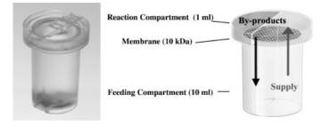
**Fig. 1.7** Device of the RTS 500 format using the Continuous Exchange Cell-Free principle.
