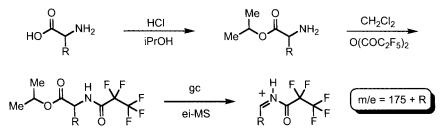
**Fig. 1.1** Most common derivatization of amino acids for GC-MS analysis. The fragment without the carboisopropoxy group normally produces the
