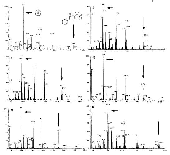
**Fig. 1.2** EI mass spectra of derivatized phenylalanine, isolated from *S. obliquus*; **a** unlabeled, **b** random 50%  $^{2}$ H-, **c** random 70%  $^{2}$ H-, **d** 100%  $^{2}$ H-, **e**  $^{13}$ C,  $^{15}$ N-, and **f**  $^{13}$ C,  $^{15}$ N/random 75%  $^{2}$ H-labeled.
